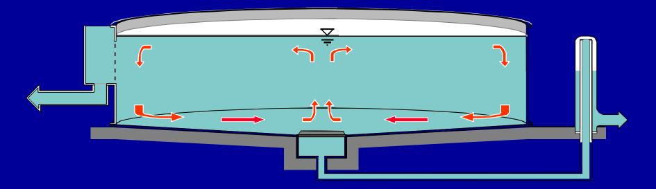
• Primary rotating flow creates secondary radial flow:
